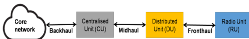
Figure 1. Mobile access network.
